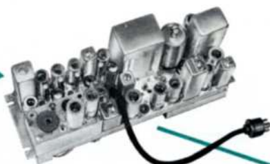
The "Building-Block" receiver chassis. Interchangeable between mobile and station combinations.
