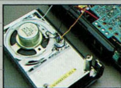
Separate speaker and electret microphone for loud and clear reception you'd expect only in larger, more expensive units.
