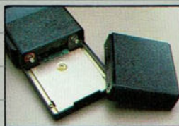
Snap-in battery is easy to replace and small enough to let you carry a spare.
