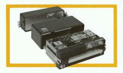
For use in relatively low noise areas such as office, fire towers and emergency communication centers, an internal switch reduces the audio power from 1.5 watts to 100 milliwatts, thus extending battery life.
