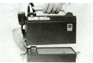
Your Porta-Mobil can be transferred from one power pack to another by releasing the retaining snap-locks, separating it from the pack, reseating it on another and re-securing the snap-locks. It takes only seconds.
