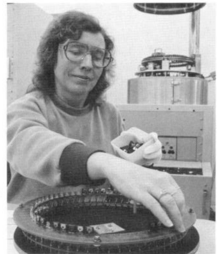
Gladys Martin loads crystals into a carousel for their final plating in the plating machine (background). Sufficient metal is plated on each side of the crystal blanks to bring them up to their operating frequency.
