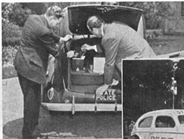
EFFICIENCY OF RADIATION IS RAISED ABOUT 40 PER CENT AND PATTERN IS MADE CIRCULAR BY MOUNTING ANTENNA ON CAR ROOF. 34-OHM CONCENTRIC LEAD TO ANTENNA IS INSTALLED AT FACTORY DURING ASSEMBLY OF THE CONNECTICUT PATROL CARS
