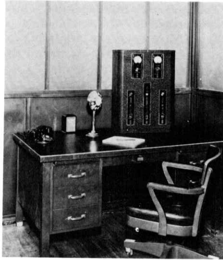
GE 50-watt ultra-high-frequency police station-house radio transmitter, in typical installation. 1936.
