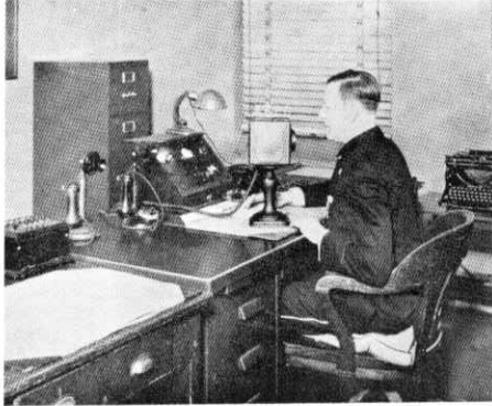
Close-up view of St. Louis Police Department's RCA radio dispatch desk with condenser microphone and transmitter control unit. (1932).
