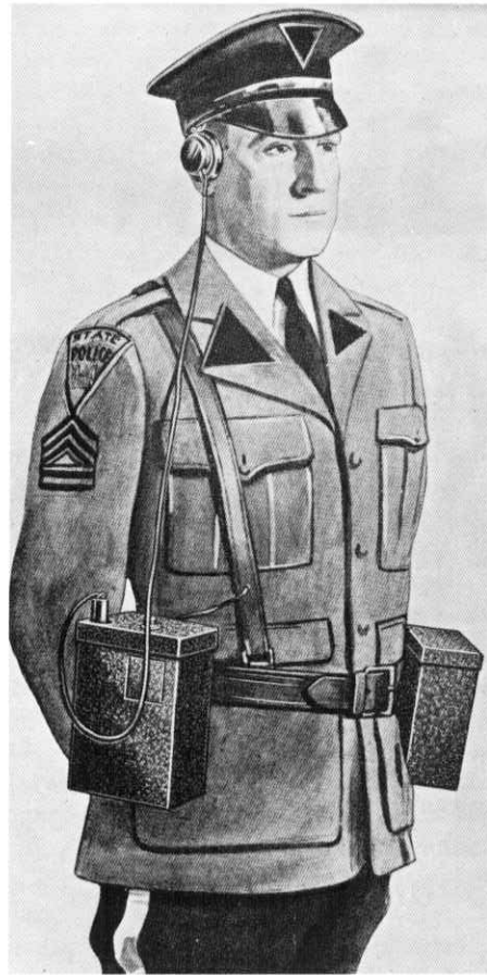
First practical "belt radio" was unveiled by RCA in 1933. Receiver is on left, battery pack on right. Antenna was encased in shoulder strap.
