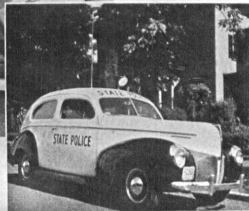
EFFICIENCY OF RADIATION IS RAISED ABOUT 40 PER CENT AND PATTERN IS MADE CIRCULAR BY MOUNTING ANTENNA ON CAR ROOF. 34-OHM CONCENTRIC LEAD TO ANTENNA IS INSTALLED AT FACTORY DURING ASSEMBLY OF THE CONNECTICUT PATROL CARS
