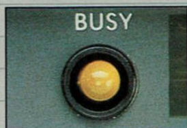
Busy light indicates that the channel is in use.
