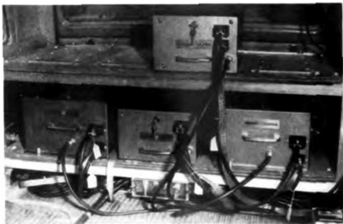
Fig. 5D: Test car equipment racks in rear of station wagon
