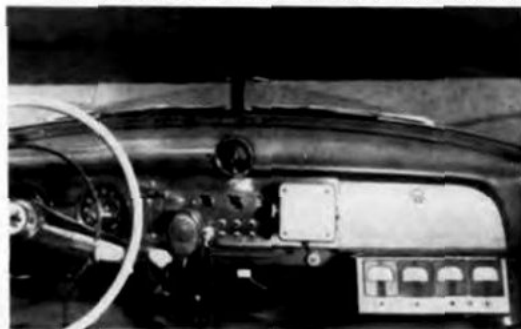
Fig. 5B: (left) Dash panel with (l to r) selector switch, transfer switch, speaker, and meter below Fig. 5C: (right) Bracket for control boxes.
